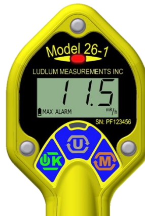
Figure 6: MAX mode operation display with ALARM indicator and alarm LED.
