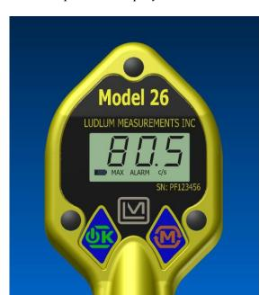
Figure 2: MAX mode operation display with ALARM indicator.
