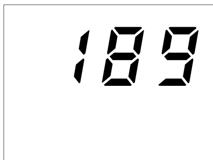
Figure 2.4: Startup Display Showing 189 Stored Data Records
