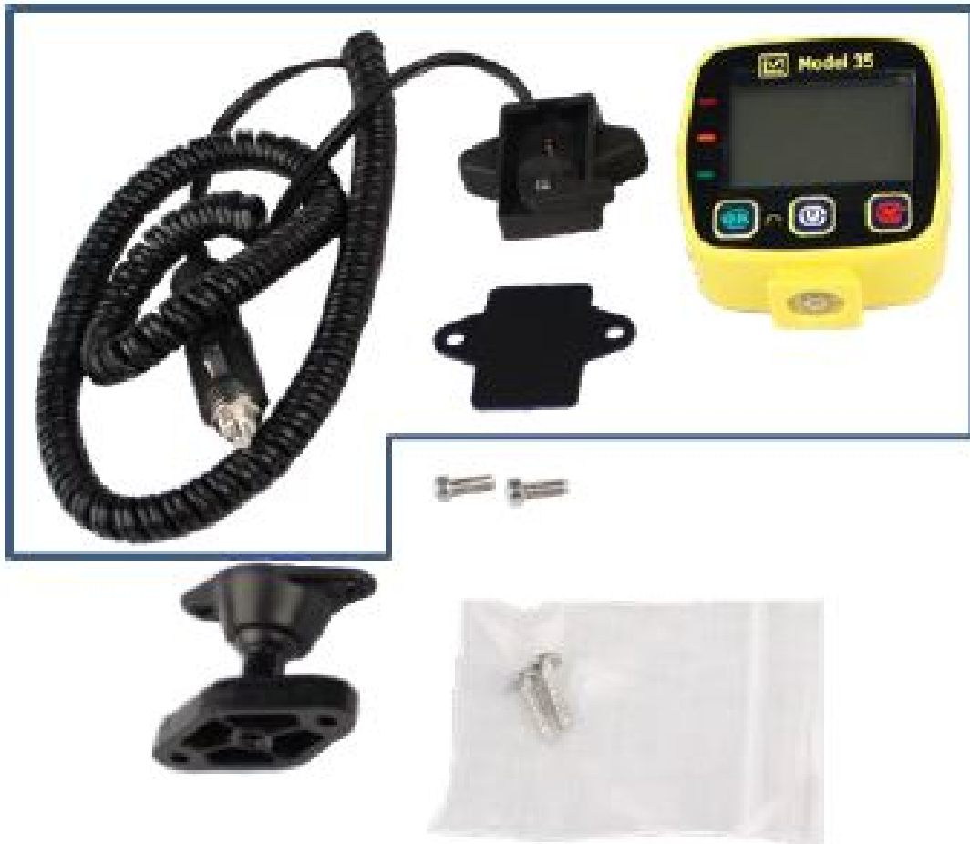
Figure A.5: Window Mount - Parts reused from disassembled shoe.
